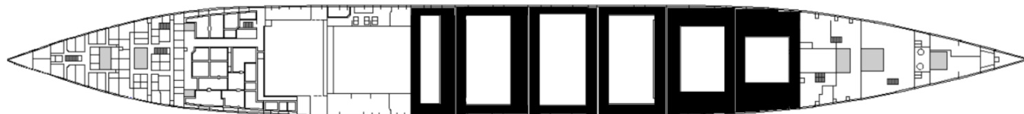
G Deck bunkers (coal stowage in black) Credit: Shipbuilder 1911(highlights by author)
