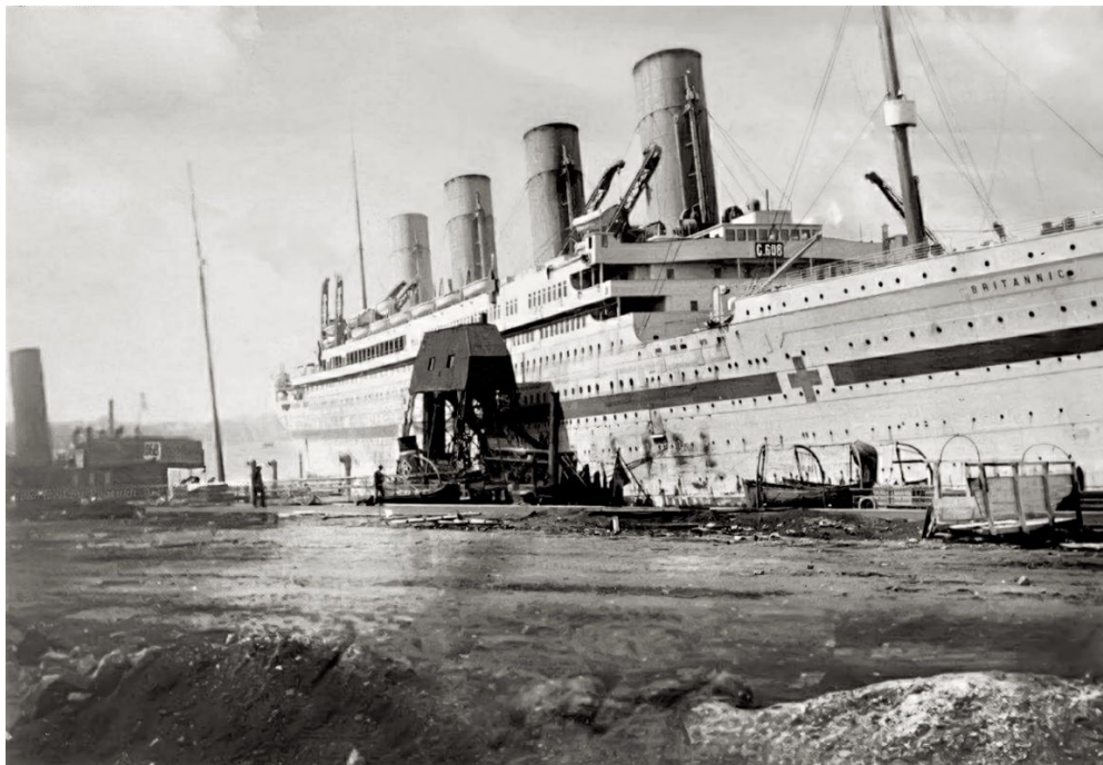
Titanic's sister, HM Hospital Ship Britannic, loading coal in Naples from a mechanized barge Credit: Wikimedia Commons
