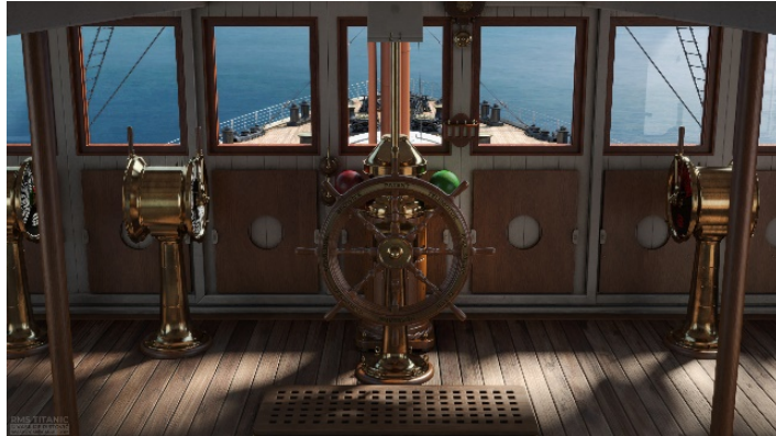
Bridge steering station - image credit: Wartsila Manufacturing
